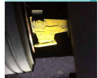
Left Hand Side front wheel (lock pin bent and slightly touching the disc)
